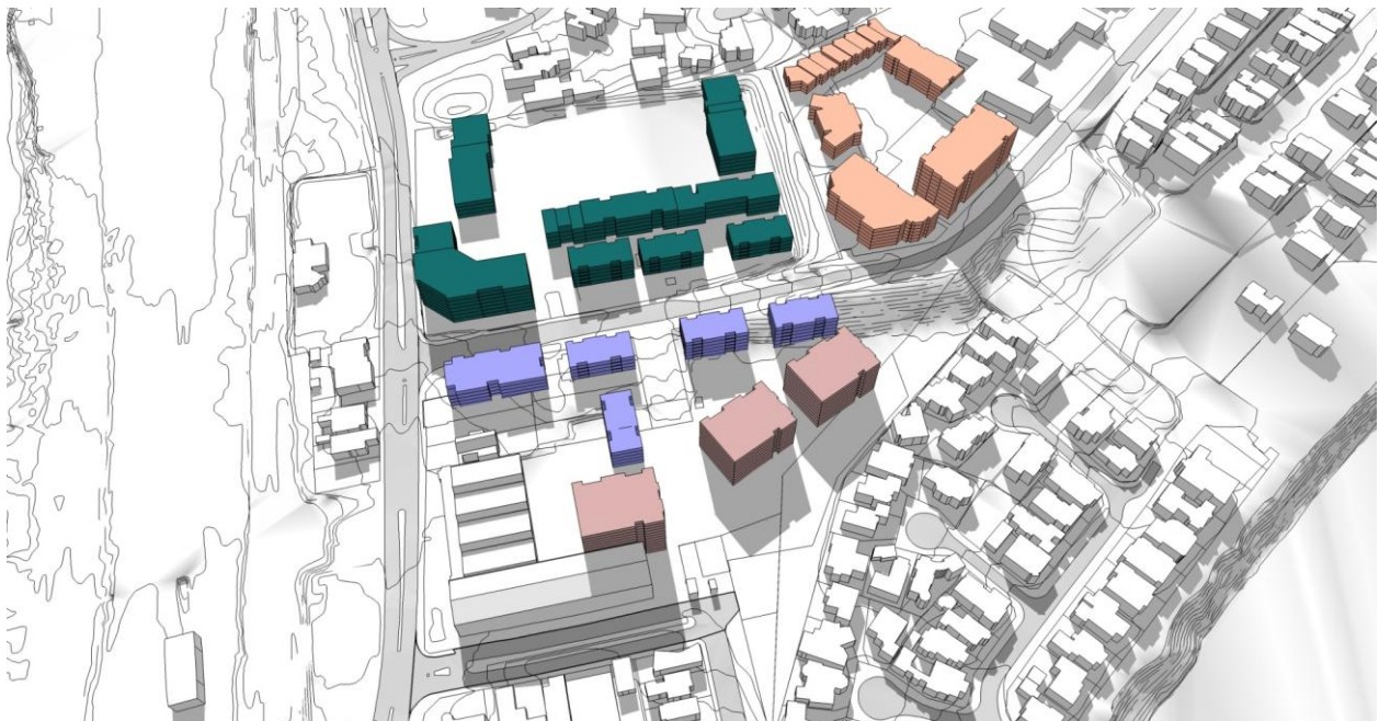
Figure 3. Shadowing of maximum discretionary building heights proposed in the review of the policy including 25m in zone D2, 33m in zone H2 and 25m in zone H3 - Officers Recommendation
