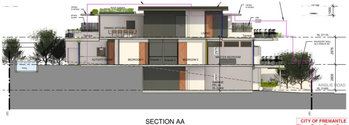
Figure 2. Section plan that shows the stepping back of the upper floor from the street boundary and floors below.
