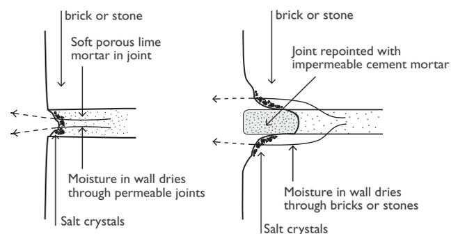
*Behaviour of mortar joints in limestone: left diagram shows a traditional permeable lime mortar, and the right diagram shows after repointing with an impermeable cement mortar. Salts crystallise where the moisture evaporates from the wall, decaying the lime mortar at left and the stones at right. It's much cheaper and easier to replace mortar than it is to replace stones. Repointing mortars should always be more permeable than the stones (or bricks).*
