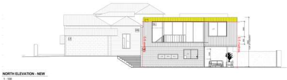
Figure 2 - The yellow highlighted section depicts the area that is non-compliant with the height limit
