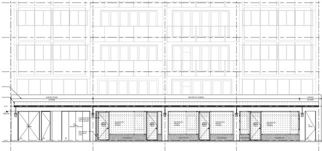
**Figure 1 –** Elevation showing the proposed 'decorative privacy screen' on the ground floor of the Serviced Apartments'
