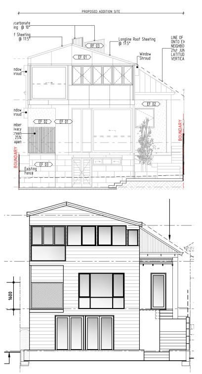
Figure 6. Approved west elevation (top) and Amended West Elevation (bottom).
