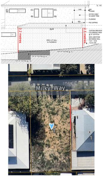
Figure 2 – Height and location of proposed boundary wall.
