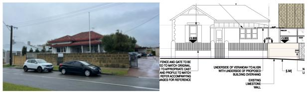
Figure 8 – Existing primary street fencing (left) and proposed (right)
