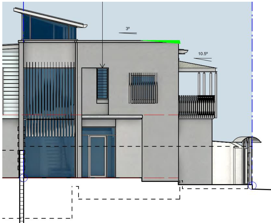
Figure 4: Portion of western wall which exceeds height requirements for walls with concealed roofs.
