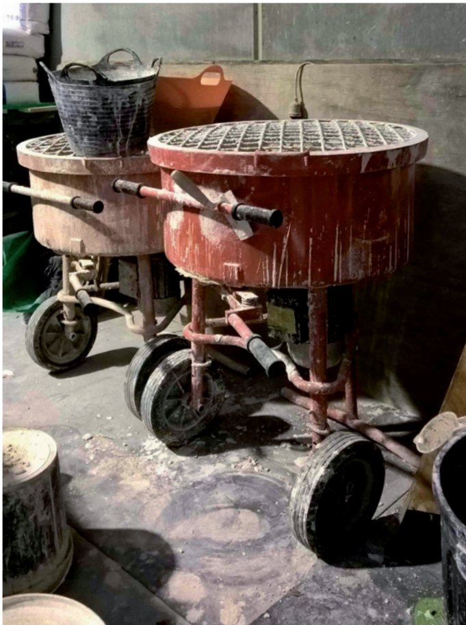
Forced action (screed) mixers. These have small blades rotating around a vertical shaft. (Photograph: Piero Casellati)
