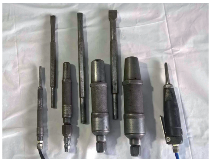
Small pneumatic hammer tools can be used judiciously to remove hard pointing. (Photograph: Piero Casellati)
