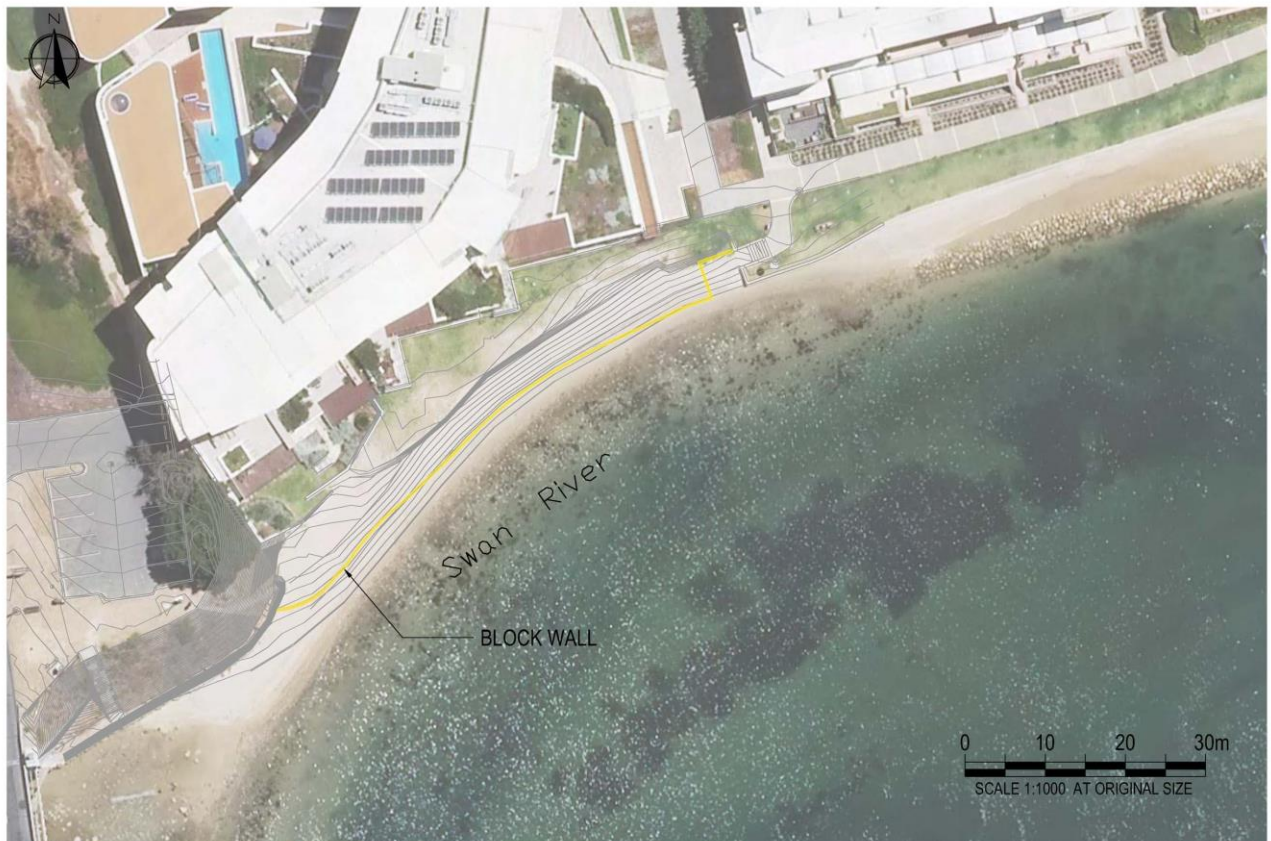
OPTION 1 A- BLOCK WALL - NO BEACH STABILISATION
