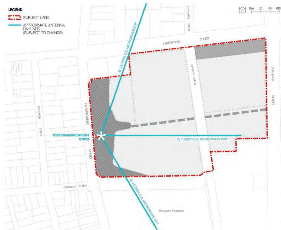
Figure 7 – Telecommunications Tower Antenna Microwave Paths
