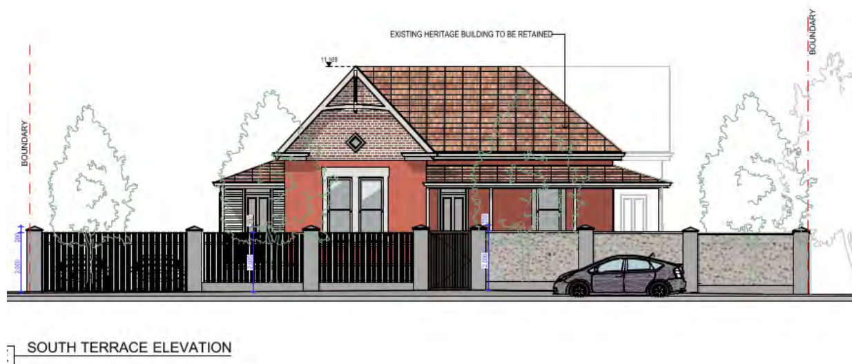
Figure 1 – Proposed primary street fencing (South Terrace)
