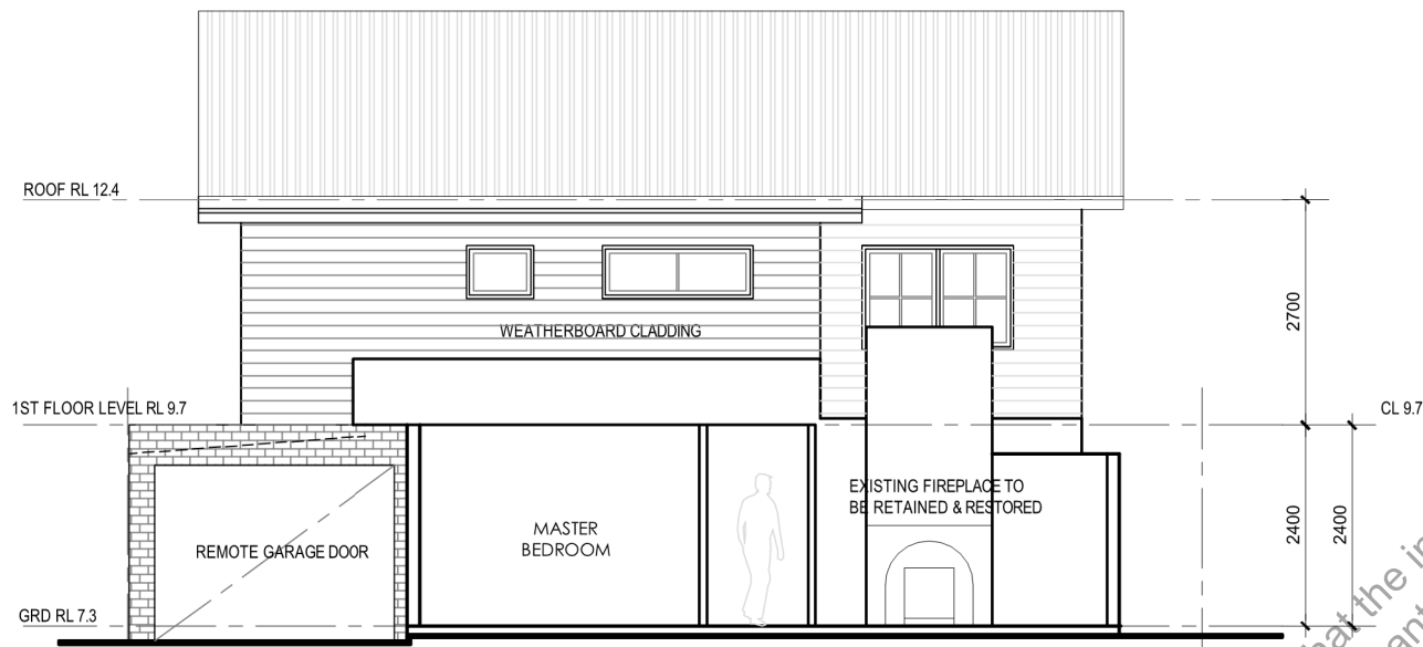
NORTH ELEVATION (UPPER FLOOR ADDITION)
