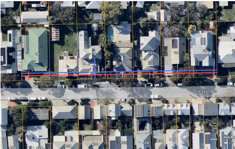
Figure 3 – Existing ground floor (red) and upper floor (blue) street setbacks within the prevailing streetscape
