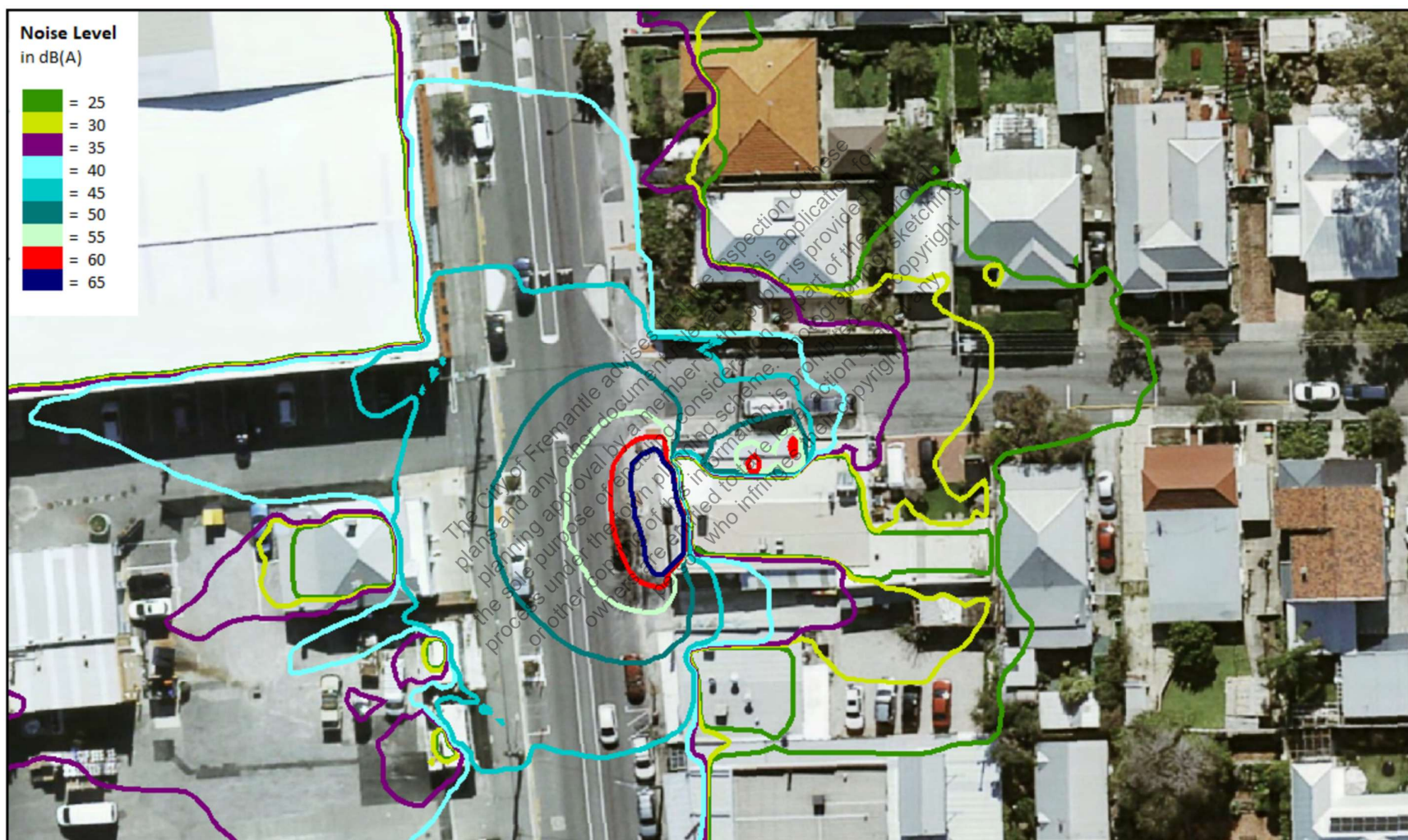
Figure 8: Worst-case night-time noise contours for scenario 2A.
